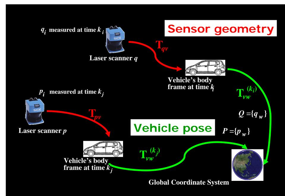
If we know sensor geometry and vehicle pose, we can integrate all laser measurements into a global coordinate system
